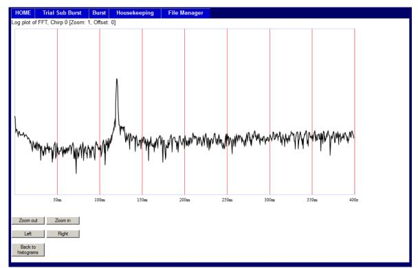
Click on the histogram with optimal characteristics, and wait (about 10 seconds – it's a slow processor...) until the browser displays a range plot of the chirp. The plot can be zoomed and panned using the buttons at the bottom of the screen. The maximum (default) depth for this plot was set on the Trial Sub-Burst page.
