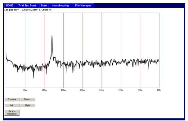
Click on the histogram with optimal characteristics, and wait until the browser displays a range plot of the chirp. The plot can be zoomed and panned using the buttons at the bottom of the screen. The maximum (default) depth for this plot was set on the Trial Sub-Burst page.
