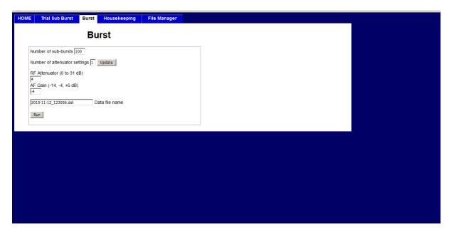
After the burst is complete, the data file will be downloaded via the browser to the computer's filing system. A copy is retained on the SD card, under a sub-directory named "survey". If a failure occurs during download, the copy will have already been safely stored on the SD card during burst acquisition. Data from Trial Sub-Bursts are discarded.
