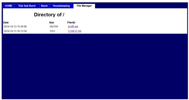
suit the desired settings, and then uploaded onto the SD card. The radar should then be switched off, the Ethernet cable disconnected, and the instrument then turned on again, when it will start up in unattended mode. The operation of the instrument is then determined by the contents of the config.ini file.
