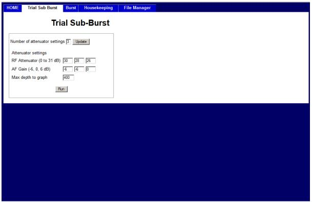
4), followed by <update>. Fill out the attenuation values – see the later section discussing criteria for the selection. Click <Test>. The PLL light on the side of the instrument will light while the various chirps are being performed (up to 4). Four histogram panels will be displayed. The histogram will indicate the dynamic range of the analogue to digital converter (ADC) that is being occupied by the
